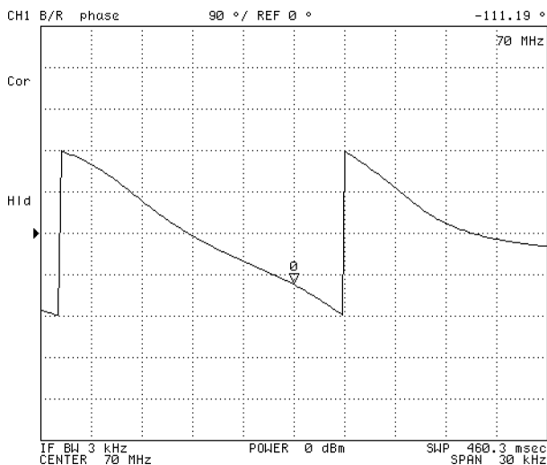
Before Adding the Electrical Length
